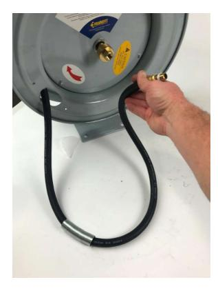
Pull at least 3 ft of hose through the reel to allow for hose twisting during assembly.
