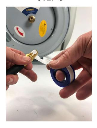
Wrap several layers of thread seal tape around the threads of the new hose.
