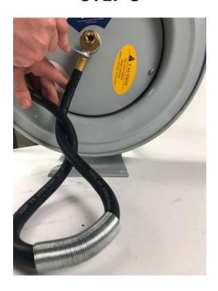
Using 14mm wrench, attach hose to hose reel hub (clockwise).
