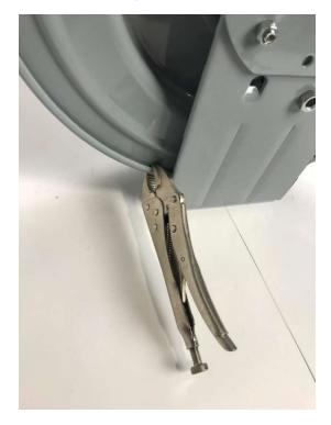
Place a secondary lock on the reel to keep it from retracting during installation by locking a vise grips on the wheel at the base as shown.
