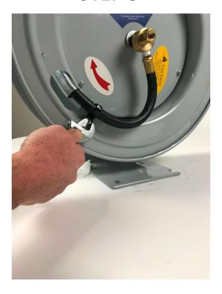
Using 8mm wrench or adjustable wrench, remove holding clamp and remove.
