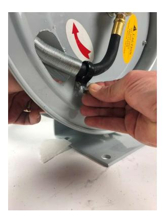
Reposition the hose protector spring into the slot in the reel wheel, then re-install the hose clamp to the hose as shown and tighten with 8mm wrench.
