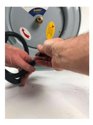
Twist hose (counterclockwise) at least 4 rotations to allow for rotation of the hose end during installation.
