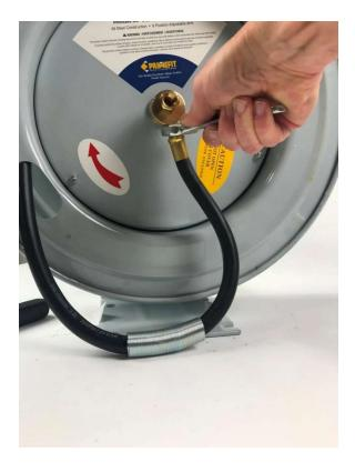
Pull some hose (approx. 3ft) through the reel to allow for twisting of the hose. Then using 14mm wrench remove the hose from the reel hub (counterclockwise).
