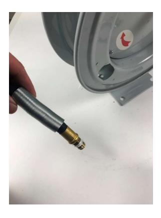
Place protective spring over the end of NEW hose prior to installing on the reel.
